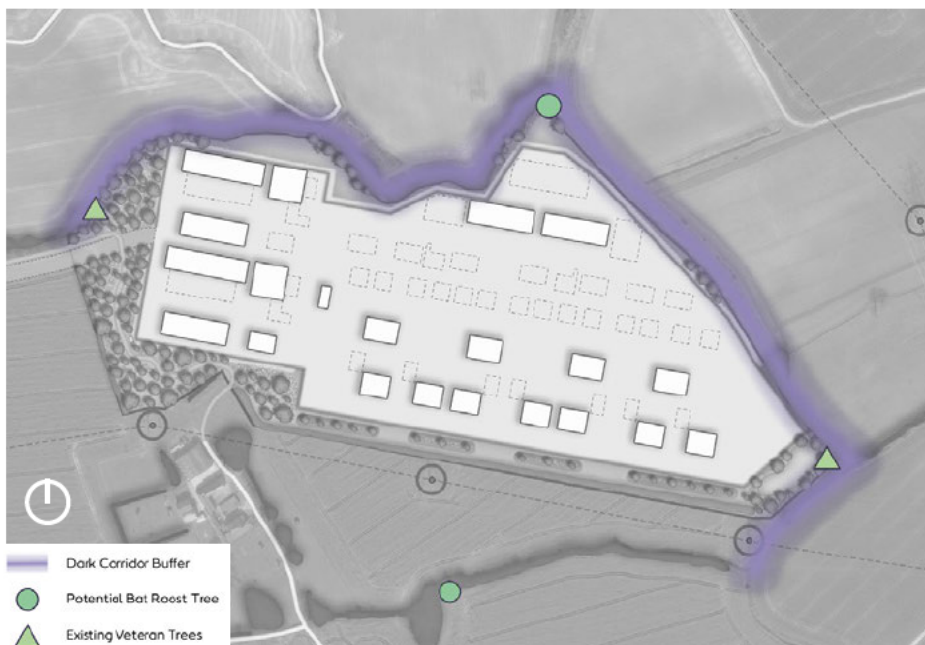
Fig 31 - Indicative plan showing dark corridor around site for wildlife movement with proposed bat roosts and existing veteran trees
